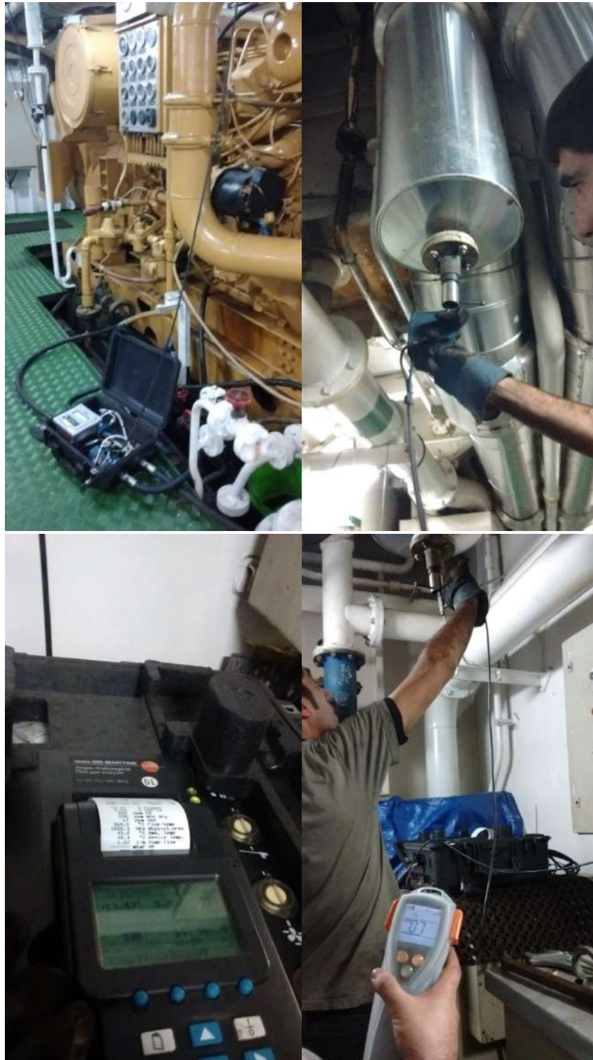
Figure 35. Emission measurement on Diesel auxiliary engines
