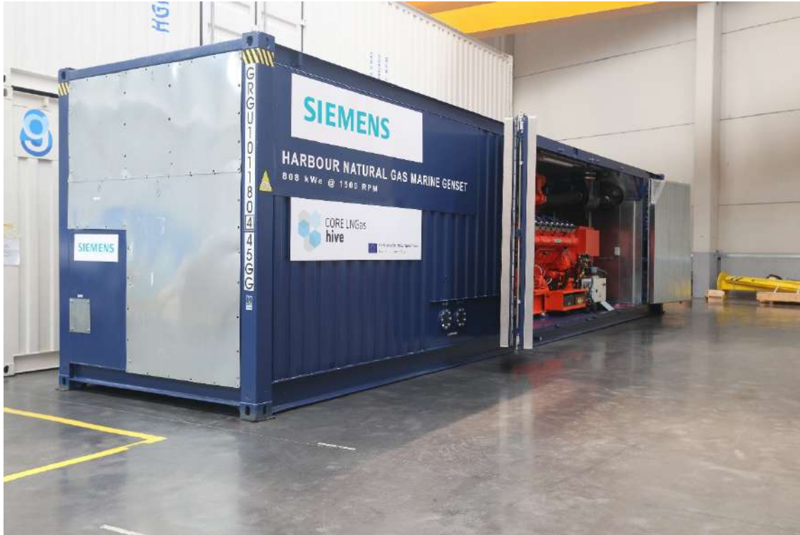
Figure 1. Module container of the LNG Genset (Siemens Engines S.A.U.).
