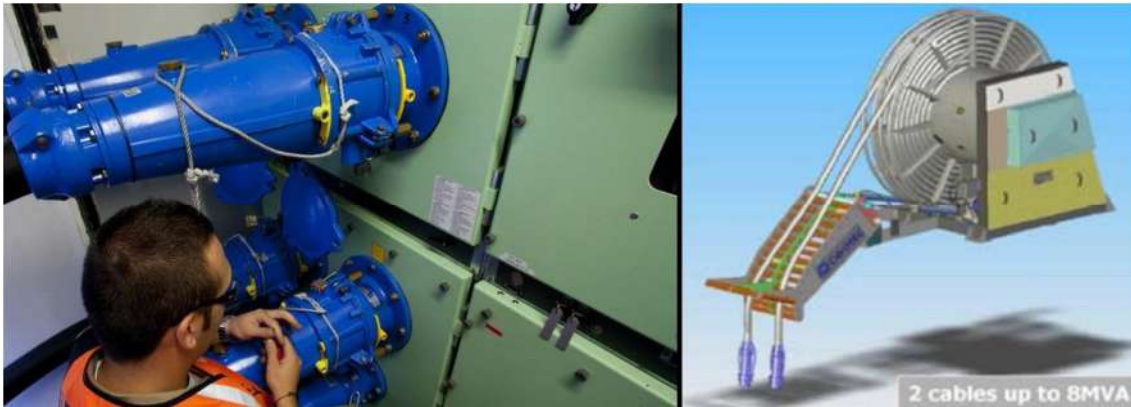
Figure 14. On board cable connection (left) and cable handling device (right)
